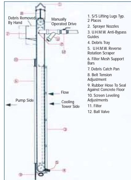
Figure 2. The traveling screen is designed to protect the process from any debris that might cause problems downstream.
